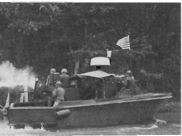
(Above) A PBR Mk II moves up a waterway in the Mekong Delta. The main visual difference between a Mk I and Mk II PBR was the curved portion of the superstructure on the Mk II. The round object atop the pole is a Raytheon 1900/W radar unit used for night patrols. (US Navy)
