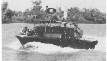
(Above) A PBR Mk II moves up a waterway in the Mekong Delta. The main visual difference between a Mk I and Mk II PBR was the curved portion of the superstructure on the Mk II. The round object atop the pole is a Raytheon 1900/W radar unit used for night patrols. (US Navy)
