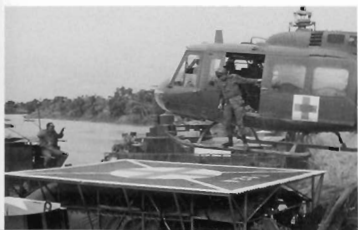
Speedy evacuation of casualties could mean the difference between life or death for the wounded. This medivac Huey comes in for a landing atop a specially modified troop carrier. These modified troop carriers were given the designation ATC(H) and often provided full medical assistance for wounded until they could be evacuated to more sophisticated facilities. (US Navy via Cressman)
